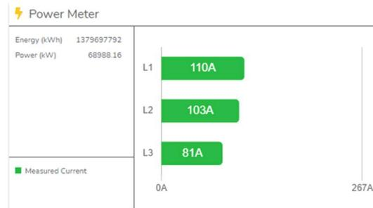
The power meter tab displays the real consumption measured by the PM, for each phasis. This consumption concerns:
