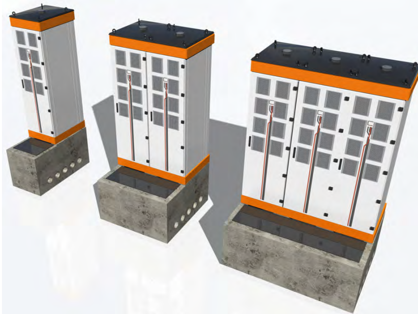
Figure 76. Example of concrete foundation (triple cabinet)
